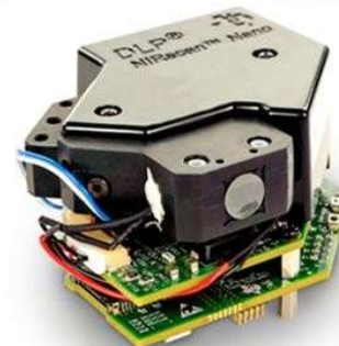
DLPNIRNANOEVN - Award winning compact battery-operated development kit for portable near-Infrared spectroscopy solutions Image 1 of 3
